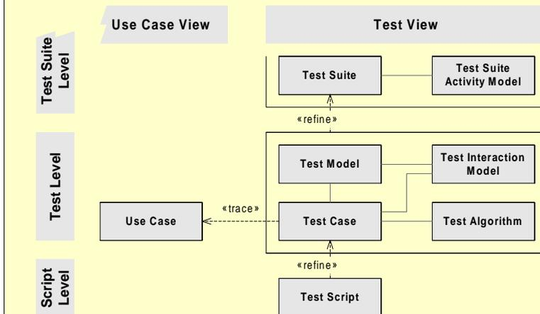
The *test view* describes the design of the software tests at different levels of granularity.
