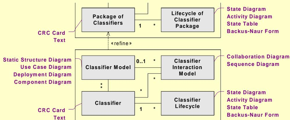
The *classifier model* specifies static relationships between classifiers. The classifier model can be represented by a set of static structure diagrams (if classifiers are subsystems, classes or interfaces), a set of use case diagrams (if classifiers are use cases and actors), a set of deployment diagrams (if classifiers are nodes) and a set of component diagrams in their type form (if classifiers are components).
