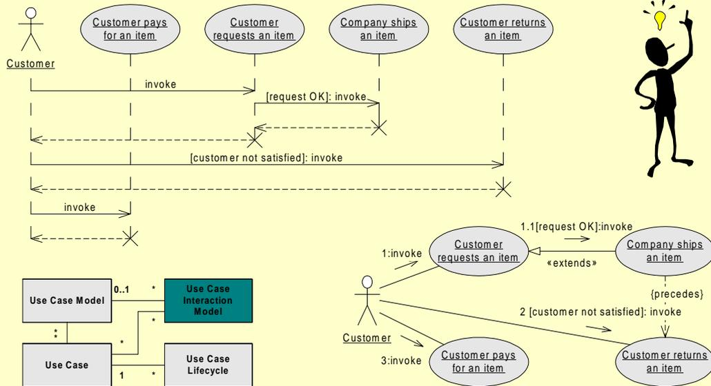
Use case interaction diagrams are sequence and collaboration diagrams in which classifier roles are use case roles. The use case interaction diagram conforms to the UML metamodel, but it is not explicitly mentioned in the UML Notation Guide
