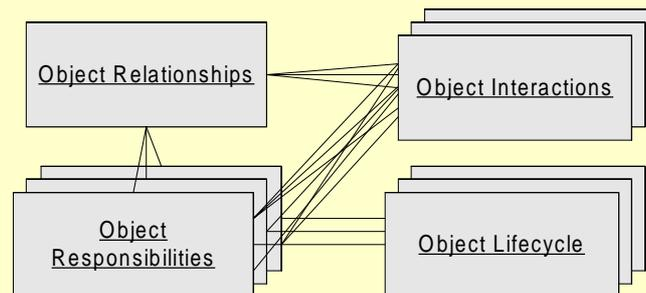
A subsystem (an instantiable package of objects) can be described by static relationships between objects, dynamic interactions between objects, object responsibilities and object lifecycles. Each of these artifacts can be represented by UML diagram or by text.
